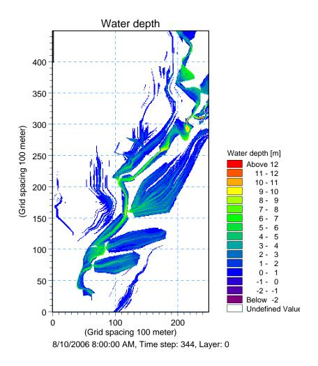
Fig. 1 Flood inundation depth map for Sabarmati basin upstream of Watrak confluence
